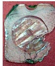
Figure 1: HEPP film after a melting and recrystallization experiment. Aluminum foils removed
