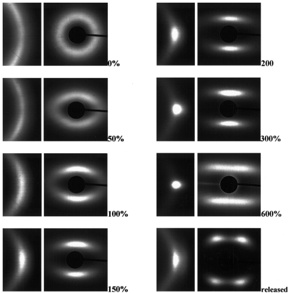
**Figure 7.** Equatorial WAXS in the angular region of the 100 pseudohexagonal and 110/200 orthorhombic reflections (left) and SAXS (right) of quenched poly(ethylene-*co*-1-octene) with 38 wt % 1-octene as a function of strain. The draw direction is vertical.
