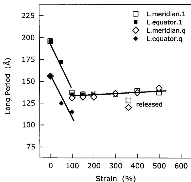
**Figure 4.** Meridional and equatorial long period of slowly cooled and quenched poly(ethylene-*co*-1-octene) with 19 wt % 1-octene as a function of strain.
