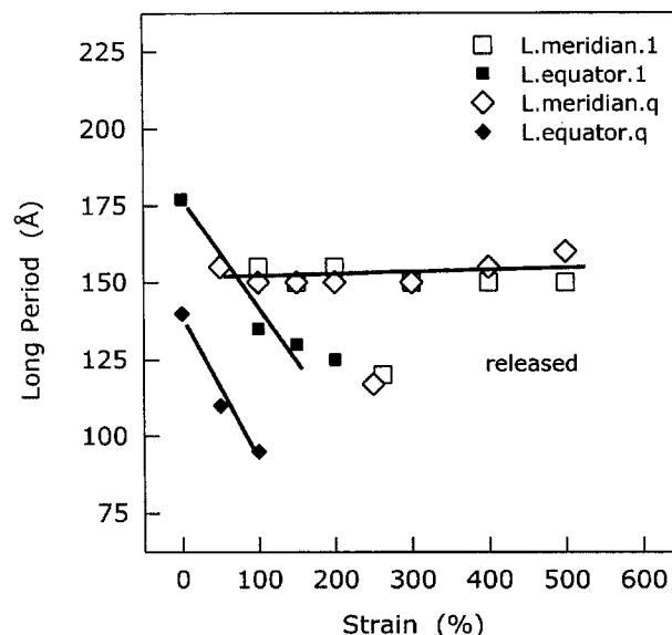
**Figure 9.** Meridional and equatorial long period of slowly cooled and quenched poly(ethylene-*co*-1-octene) with 30 wt % 1-octene as a function of strain.
