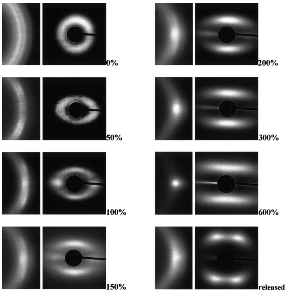
**Figure 6.** Equatorial WAXS in the angular region of the 100 pseudohexagonal and 110/200 orthorhombic reflections (left) and SAXS (right) of slowly cooled poly(ethylene-*co*-1-octene) with 38 wt % 1-octene as a function of strain. The draw direction is vertical.
