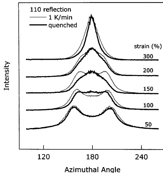
**Figure 5.** Azimuthal intensity distribution of the WAXS 110 reflection of quenched and slowly cooled poly(ethylene-*co*-1-octene) with 19 wt % 1-octene as a function of strain between 0 and 300%. The equator is at 180°.
