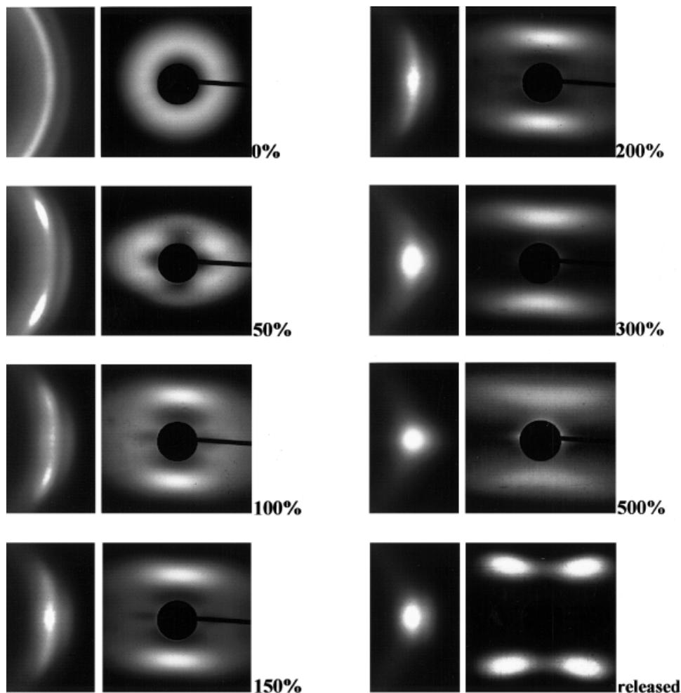
**Figure 3.** Equatorial WAXS in the angular region of the 110 and 200 reflections (left) and SAXS (right) of quenched poly(ethylene-*co*-1-octene) with 19 wt % 1-octene as a function of strain. The draw direction is vertical.
