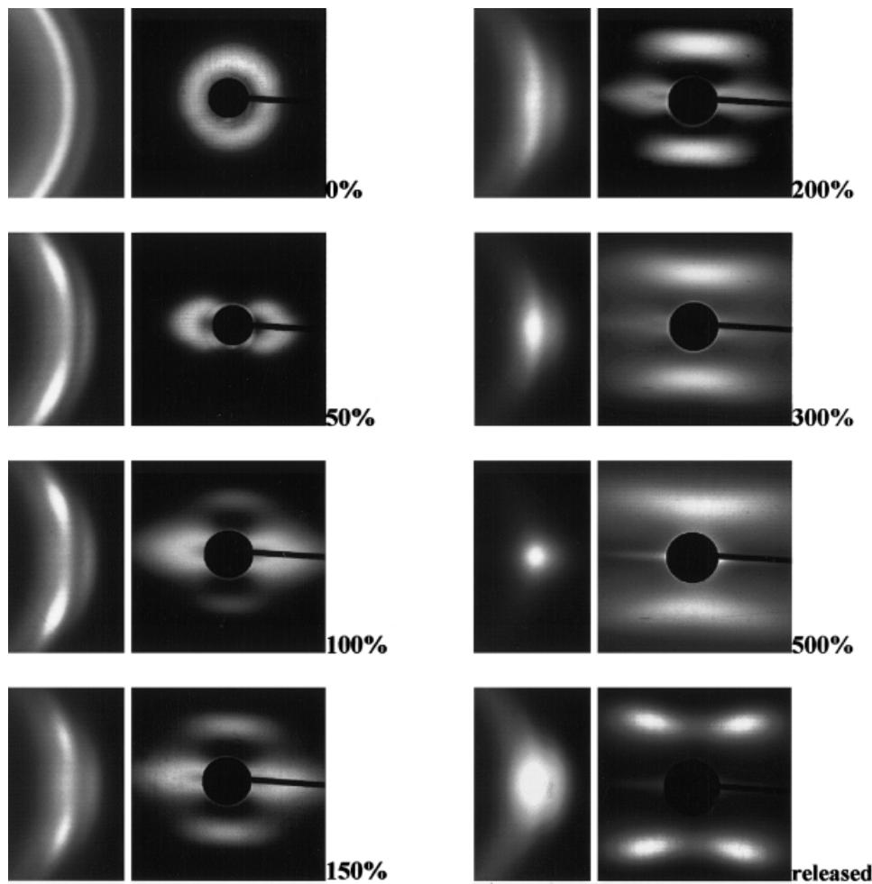
**Figure 2.** Equatorial WAXS in the angular region of the 110 and 200 reflections (left) and SAXS (right) of slowly cooled poly(ethylene-*co*-1-octene) with 19 wt % 1-octene as a function of strain. The draw direction is vertical.
