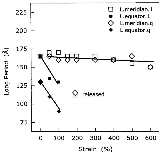
**Figure 8.** Meridional and equatorial long period of slowly cooled and quenched poly(ethylene-*co*-1-octene) with 38 wt % 1-octene as a function of strain.
