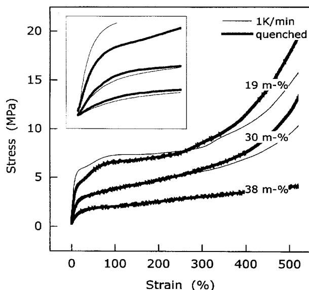
**Figure 1.** Stress-strain curves of slowly cooled and quenched poly(ethylene-*co*-1-octene) with 19, 30, and 38 wt % 1-octene.
