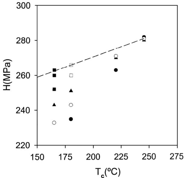
Fig. 1. Variation of microhardness  $H$ , during secondary crystallization, with crystallization temperature, for different times: (●)  $t_c = 0.5$  h, (○)  $t_c = 2-3$  h, (▲)  $t_c = 24$  h; (■, □) long  $t_c$  values (up to more than 300 h).
