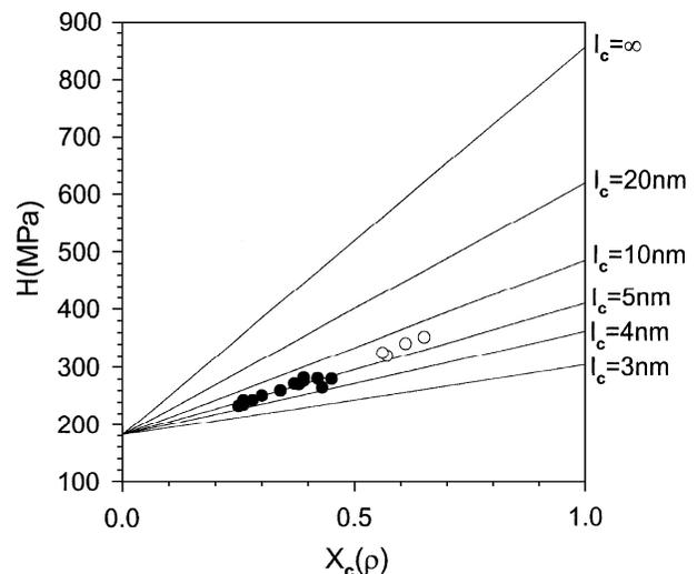
Fig. 3.  $H$  variation with  $X_c$  for atmospheric (solid symbols) and high-pressure (open symbols) crystallized PEN. The straight lines follow Eq. (7) (see text).
