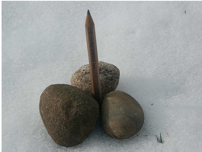
Figure 13: Model of a layer made by agglomeration in a plane of 3 differently oriented crystallites (pebbles). The plane is normal to the fiber direction (pencil)
