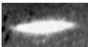
Figure 2 Digitized image of a primary beam profile at beamline A2, HASYLAB. The length of the bright spot is 3 mm
